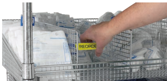
Lower Kanban Flipper to Signal to the Portal that Inventory Needs to be Replenished
