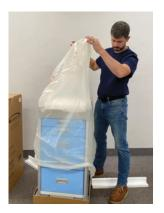
2 Remove the plastic cover over the QT Cart. **NOTE** Set packing materials to the side until you are able to test the product to ensure it is working properly.
