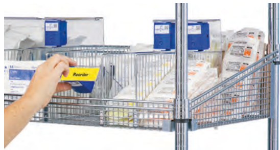
Lower Kanban Divider to Signal to the Controller that Inventory Needs to be Replenished
