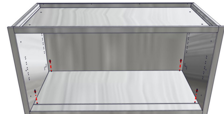
Fig 10: Remove 4 front screws
