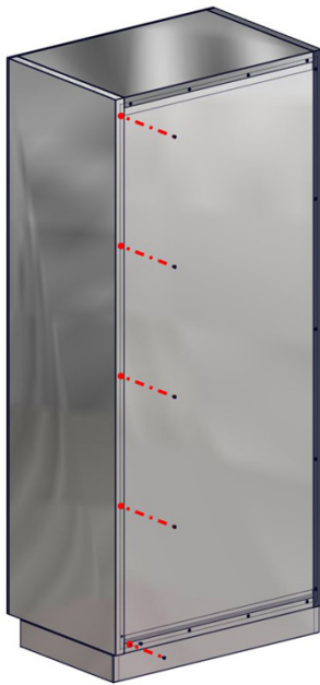
Fig. 30: Remove screws in back
