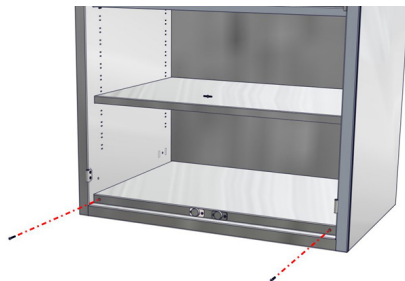
Fig. 9: Remove front screws
