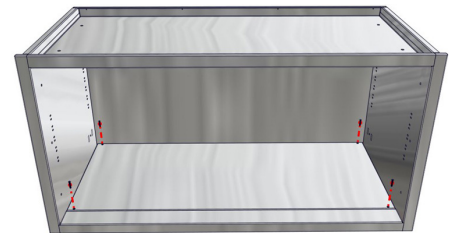
Fig 21: Remove 4 front screws
