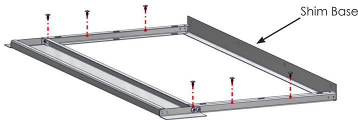
Fig. 22: Remove six interior screws
