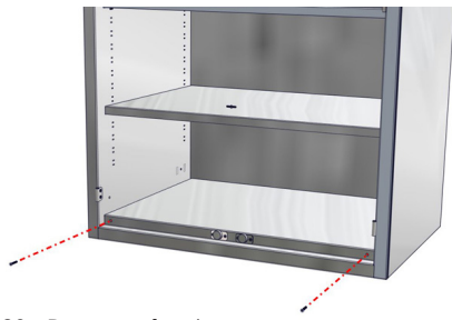
Fig. 20: Remove front screws
