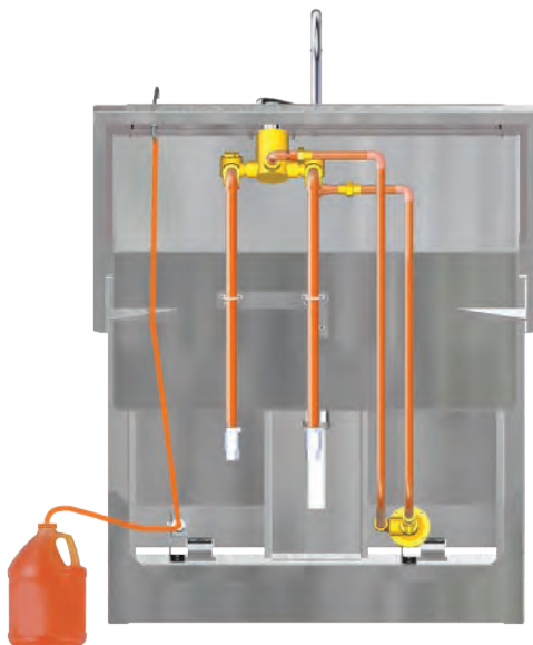
Fig. 11 - Install Soap Dispenser Tubing
