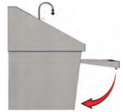
Fig. 28 - Door Should Rotate Freely on Hinges
