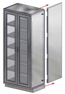
Fig. 28: Remove exterior side panel
