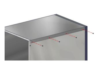
Fig. 11: Remove for screws from rear
