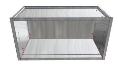
Fig. 7: Remove four screws
