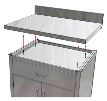
Fig. 13: Attach Work Surface
