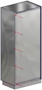
Fig. 27: Remove rear screws
