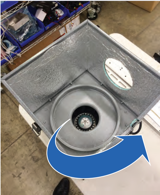
Cabin HEPA Filter Box with Top Removed Twist cap to access HEPA Filter
